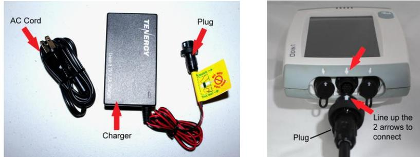
When connected to the device, plug the AC cord into the other end of the charger and then into a 110-120V outlet. At first you will see a red light on the charger. After about 3 hours it will turn a steady green color when charging is complete.
